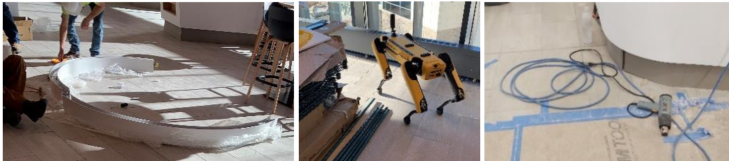
Figure 5. Presence of objects less than 11.8 inch high and cords on floor on Spot's navigation path
