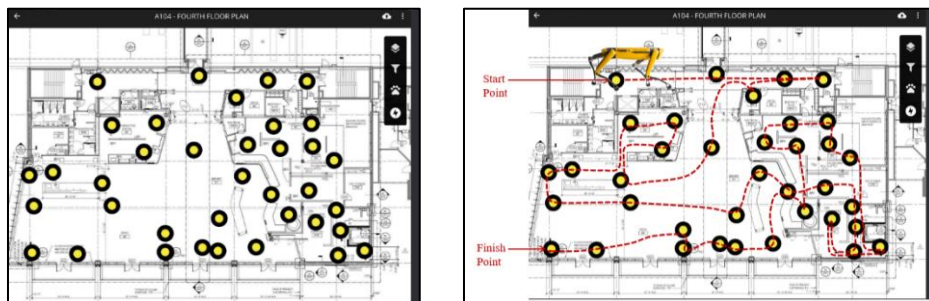
Figure 2. Left: HoloBuilder app interface with the saved waypoints for Spot saved on the 2D floor plan; Right: Spot's starting point, end point and its navigation path during the mission
