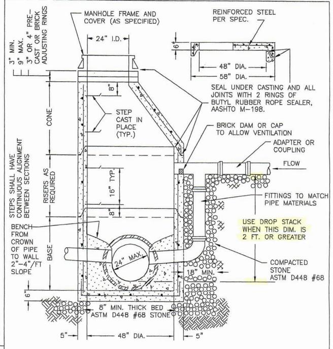
MATERIALS AND FABRICATION SHALL BE IN ACCORDANCE WITH ASTM C478 UNLESS OTHERWISE SHOWN. CONE SHALL BE OF THE ECCENTRIC TYPE. FOR NEW LINES, CONNECT PIPE TO SECTION WITH APPROVED FLEXIBLE WATER-TIGHT SLEEVE OR GASKET (INTERPACE OR THE FLEXIBLE WATER-TIGHT SLEEVE OR GASKET SHALL BE INSTALLED PER THE MANUFACTURER'S RECOMMENDATIONS.
