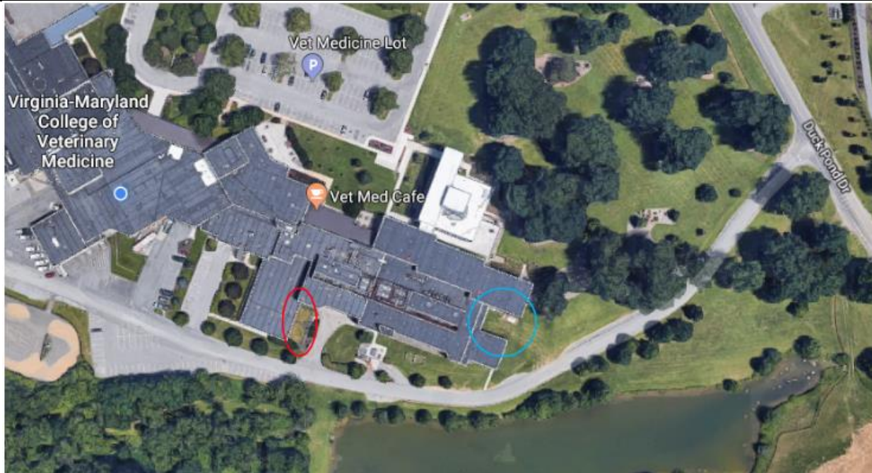
Figure 1. This aerial image shows the current location of the outdoor run (circled in red) and the proposed new location (circled in blue). This alcove is not currently used for any purpose and would make the ideal location for the new outdoor run because it is relatively flat and the building walls can be integrated into the structure, which minimizes the amount of fencing required.
